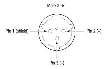
Figure 39: Standard balanced-output pin assignments
